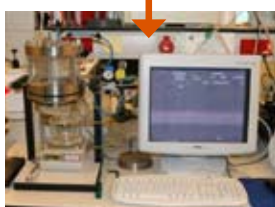
TU Delft: Bio concrete in a permeability setup
