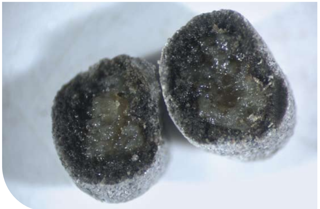
TU Delft: Capsule made of porous sand containing oil used for self healing of porous asphalt.
